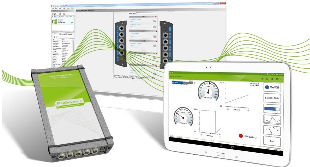
BU: With FlexConfig RBS 4.3 and the new devices of the FlexConfig family, even more complex gateways and restbus simulations are possible.
