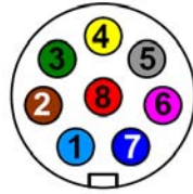
Figure 3: Front panel jack pin assignment, front view of the 8 pin Binder 712 female connector
