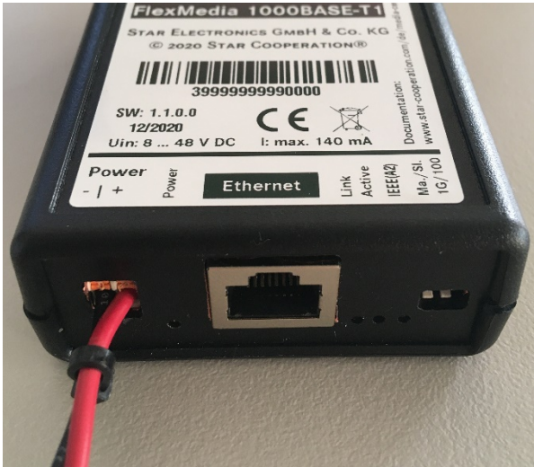
Figure 1: Side with Power and Ethernet (1000BASE-TX)
